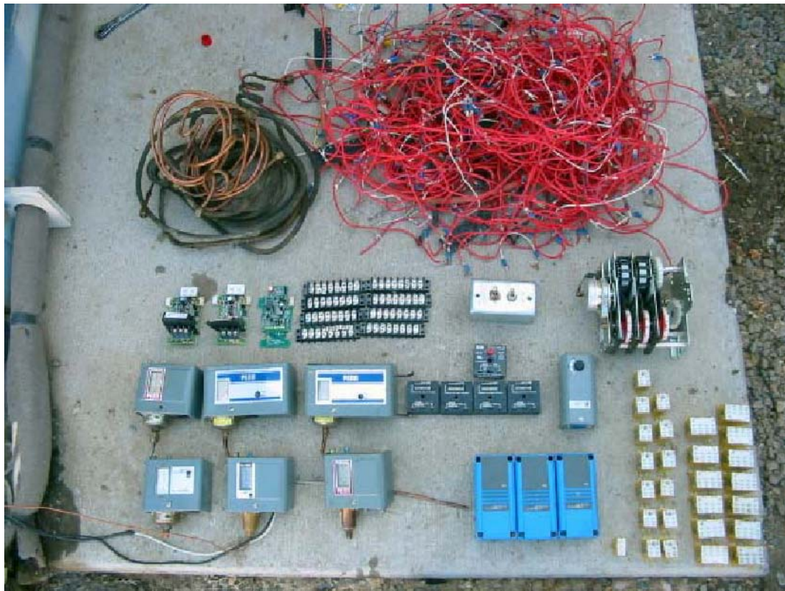
Figure 1. This assortment of pressure switches, relays, staging controls, wire, and a defrost timer were replaced by two CR-110 control cards.
